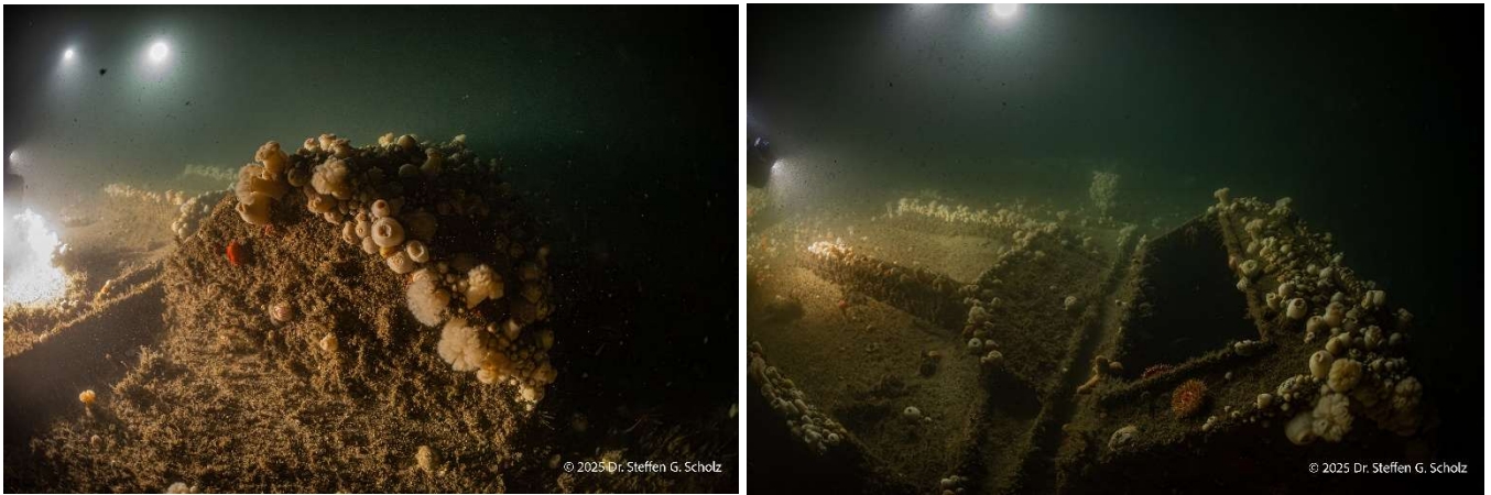
Figure 18: Skylight structure adjacent to the aft cargo hold, part of the ship's original ventilation system.
