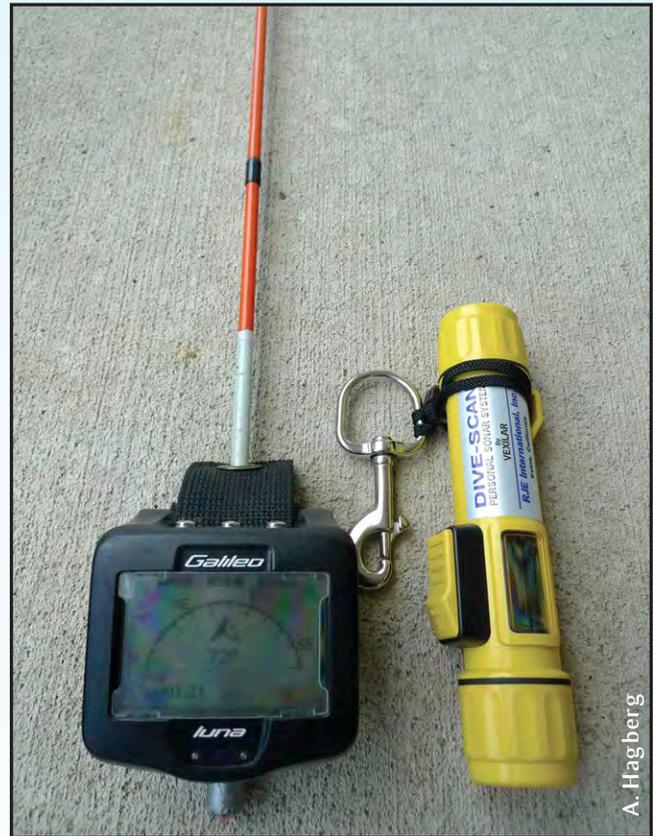
*Andreas' survey equipment (wet notes not included). The digital compass is mounted on a 2-foot stick with a marking in the middle; this reduces the guess work from a station to the nearest knot on the line. The yellow sonar measures distance, useful when measuring the width and depth of a passage.*
